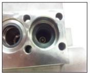
4) Note: do not grease any portion of the packing assembly during this process. Set high pressure seal insertion collar in manifold cylinder. Assemble Glyd rings (positions 5 & 6) and gently place inside cylinder tool so they are resting evenly. Insert pusher tool and firmly press down to set packing in manifold.
