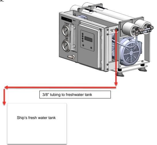
WARNING - SHIPS FRESH WATER TANK MUST BE VENTED PROPERLY TO AVOID BACK PRESSURE ON SYSTEM. FAILURE TO DO SO MAY CAUSE PERMANENT DAMAGE TO SYSTEM AND/OR TO NOT FUNCTION PROPERLY.
