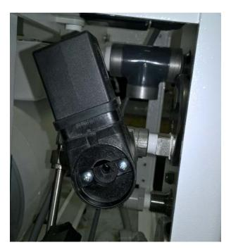
3. Adjust set point with 5/64<sup>th</sup> Allen wrench, clockwise to increase setting and counterclockwise to lower the setting.
