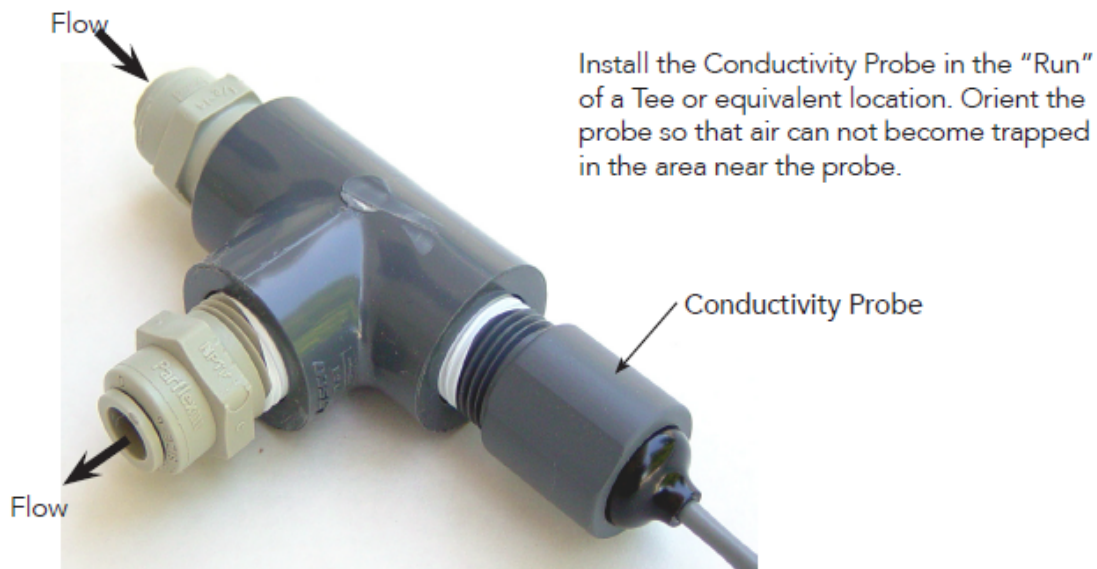
Figure 5. Conductivity Probe Installation
