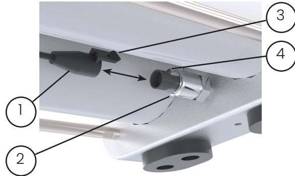
FIGURE 24: PRESSURE TRANSDUCER CAP CONNECTION
